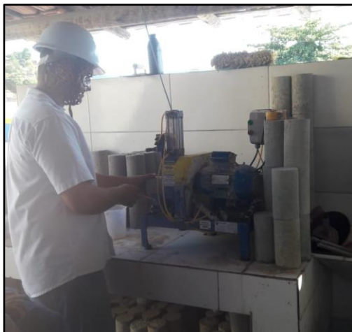
Figure 11 – Concrete specimens rectification.
