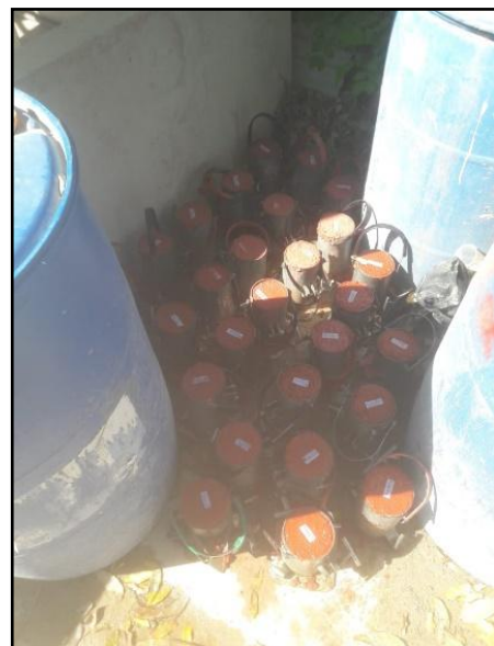
Figure 9 – Molds filled with the densely packed mixtures.
