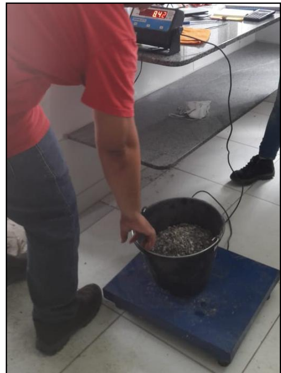
Figure 5 – Weighing of coarse aggregate for mixing concrete.
