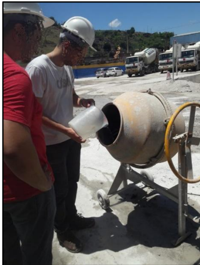
Figure 6 – Mechanical mixing of concrete constituent materials.
