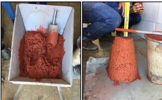
Figure 7 – On the left, a freshly colored concrete mix and on the right, a consistency measurement (Slump Test).
