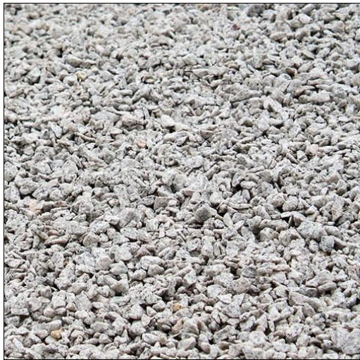
Figure 3 – Coarse aggregate (gravel 0) of gneissic origin (Grupo pedreira Mix Mattar, 2020).
