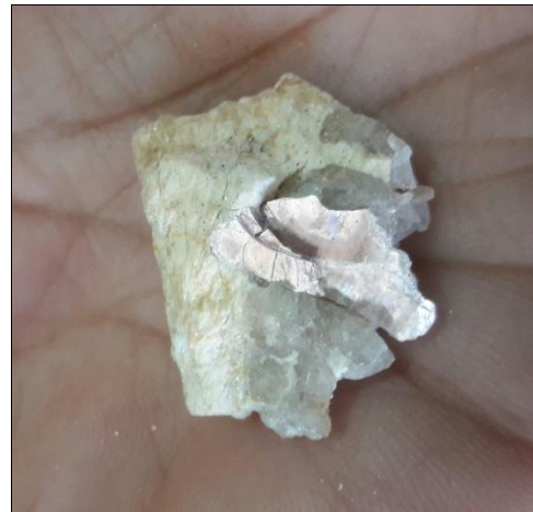
Figure 4 – Quartzite with the presence of biotite sheets in its composition.
