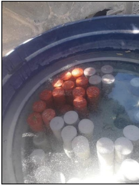
Figure 10 – Test specimens subjected to wet curing.
