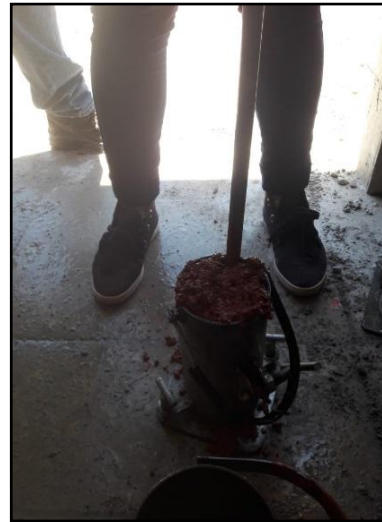
Figure 8 – Densification of the mixture in the cylindrical test specimens with the aid of the steel rod.
