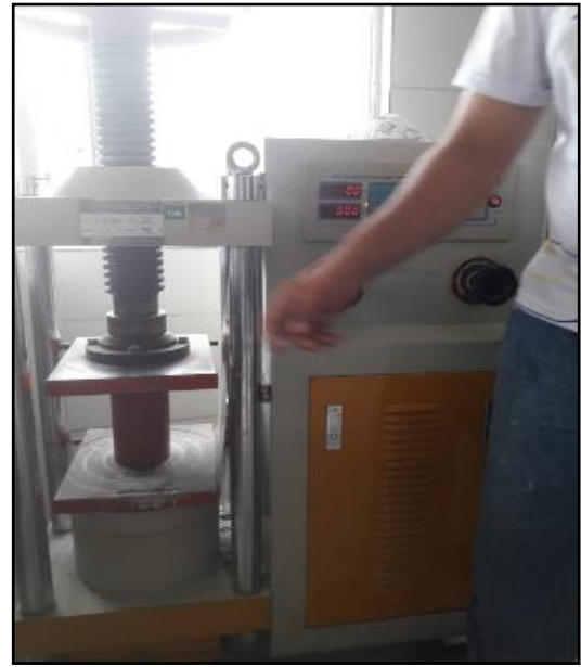
Figure 12 – Test specimen subjected to compression test in electric press.
