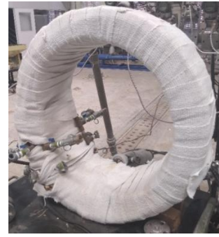
Figure 6 – Thermally insulated coil with ceramic fiber tape.
