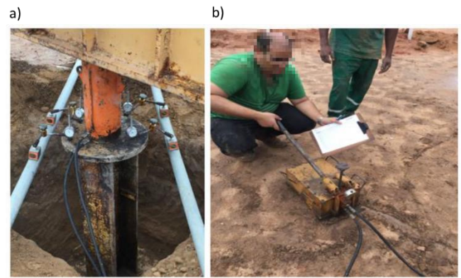
Figure 9 – a) Monometer b) Pump (helps load application).
