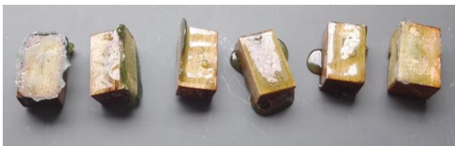
Figure 20 - Test body after melting PET 1.
