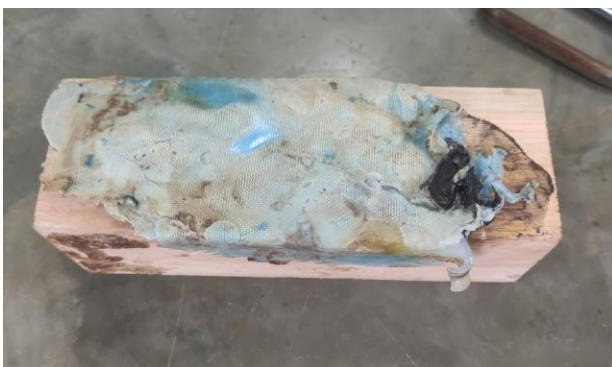
Figure 17 - Test body after molding with melted PET.
