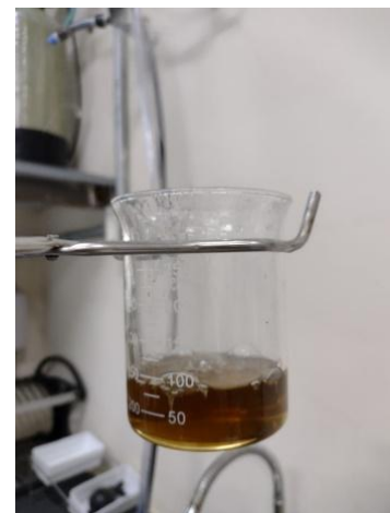
Figure 18 – Plastic resin obtained by heating glycerin with PET 1.
