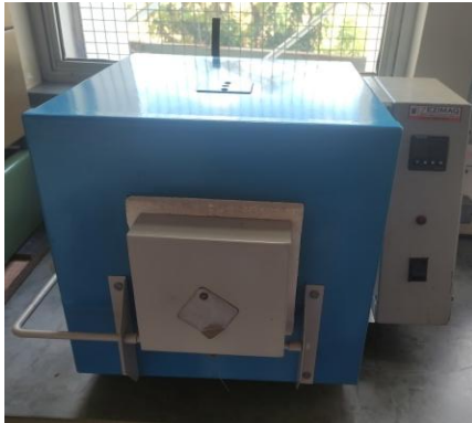
Figure 9 – Zezimaq microprocessed muffle furnace.
