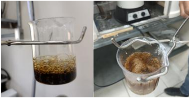
Figure 19 - Heating test glycerin with PET 1.
