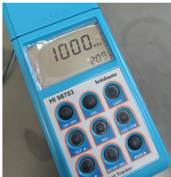
Figure 3 – Determination of initial turbidity (1000 NTU) of the prepared clay solution.
