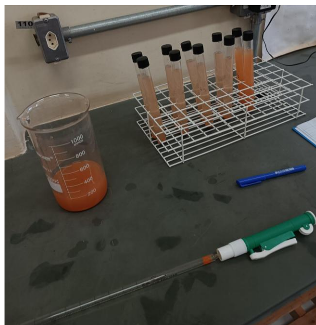
Figure 5 – Collection and reading of samples, through the experiment of turbidity decay.
