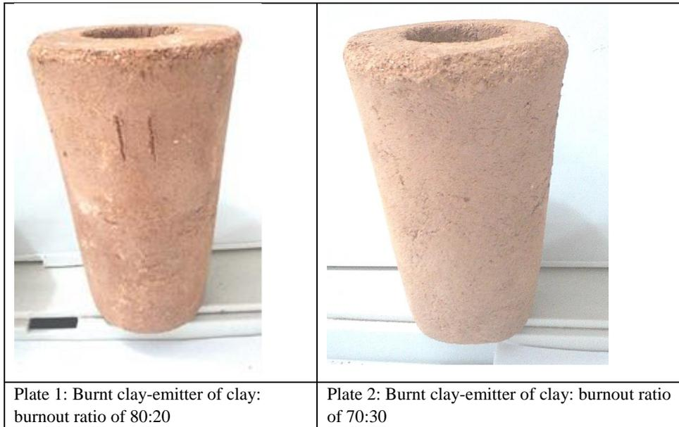
**Figure 1:** Burnt clay-emitter of clay. Plates 1 and 2.
