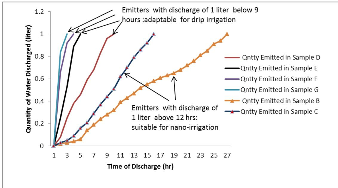
**Figure 3:** Discharge of water in clay emitters.
