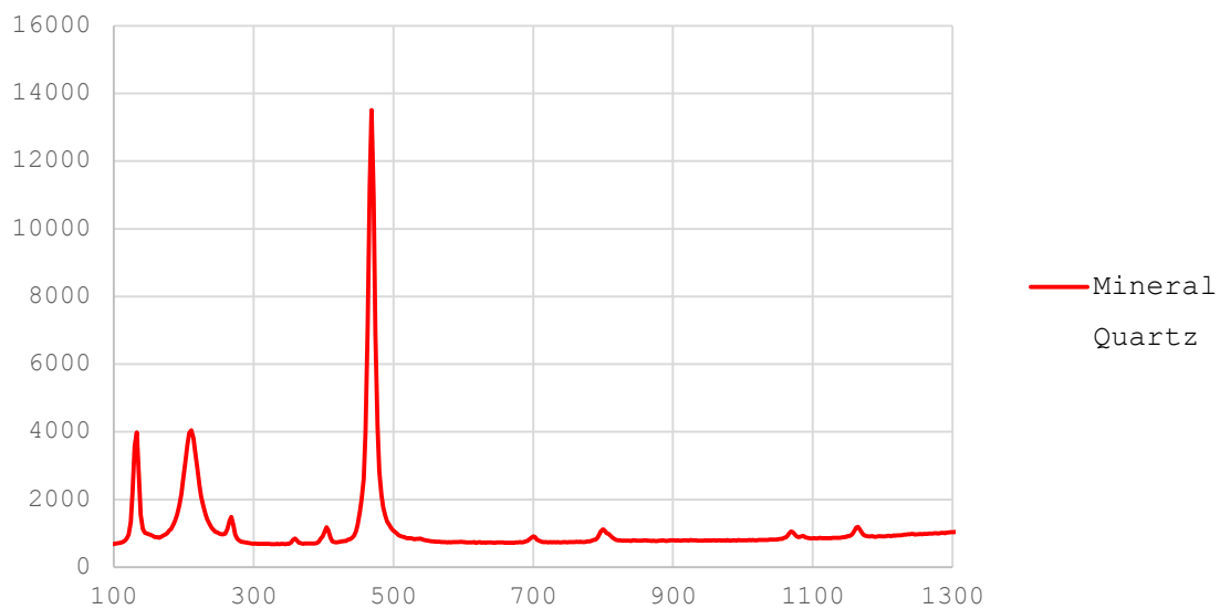
Figure S12. Graph of the Raman spectrum obtained from the mineral included in the SJ1 diamond (in red) and the spectrum of alpha quartz (R040031) from the RRuff database (in blue).
